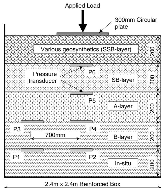
Figure 2: Laboratory test set-ups
