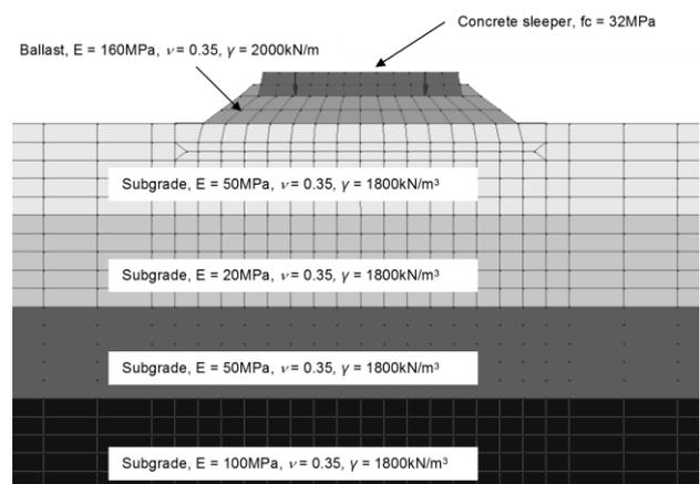
**Figure 3: Basic finite element model of track structure and substructure**
