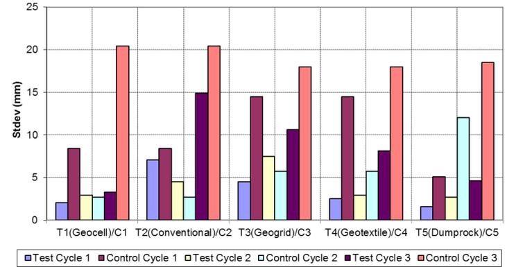
**Figure 5: Standard deviation of settlement measurements per test section**
