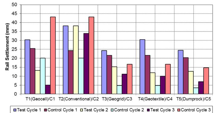
**Figure 6: Average rail settlement measurements per test section**
