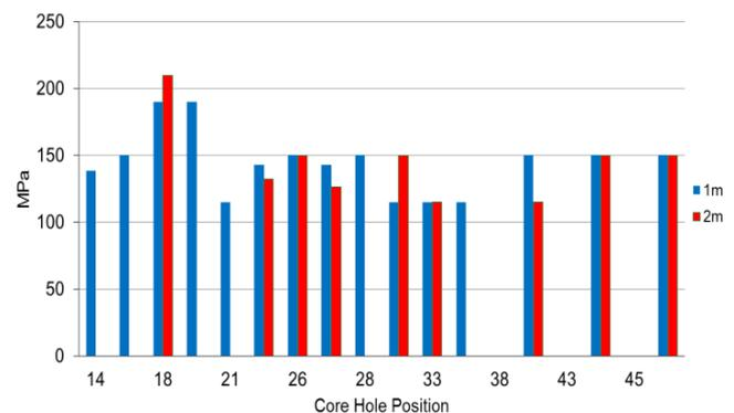
Figure 9: Typical UCS values (Beaconhill tunnel)
