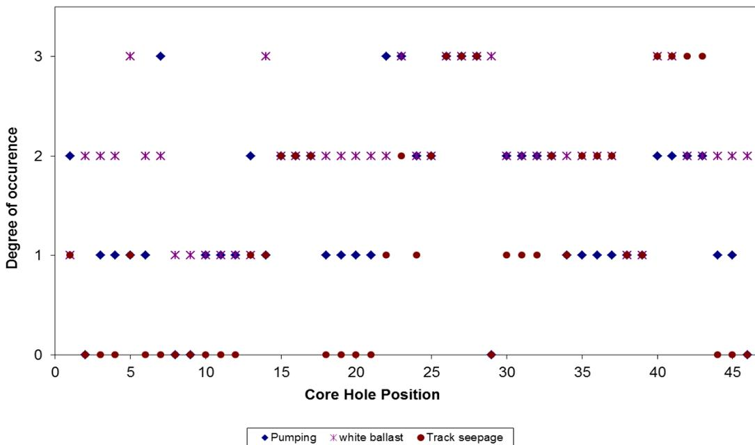
**Figure 2: Parameters observed during visual inspection and their relative distribution (Beacon Hill)**
