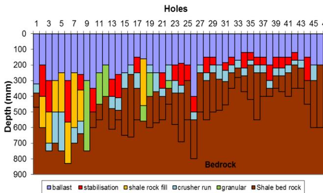
Figure 4: Typical substructure material composition
