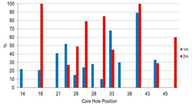
Figure 8: Typical RQD values (Beaconhill tunnel)
