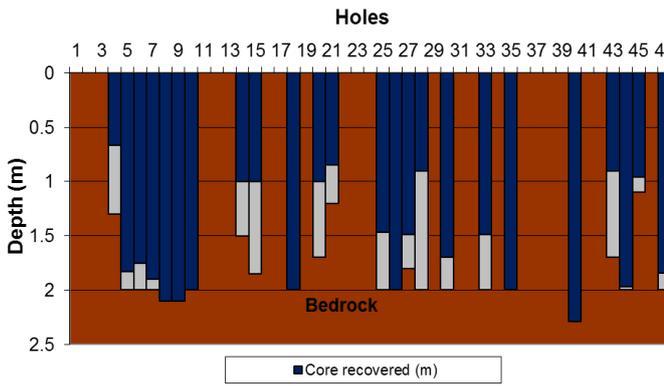
Figure 6: Positions of cores recovered (B. Hill)
