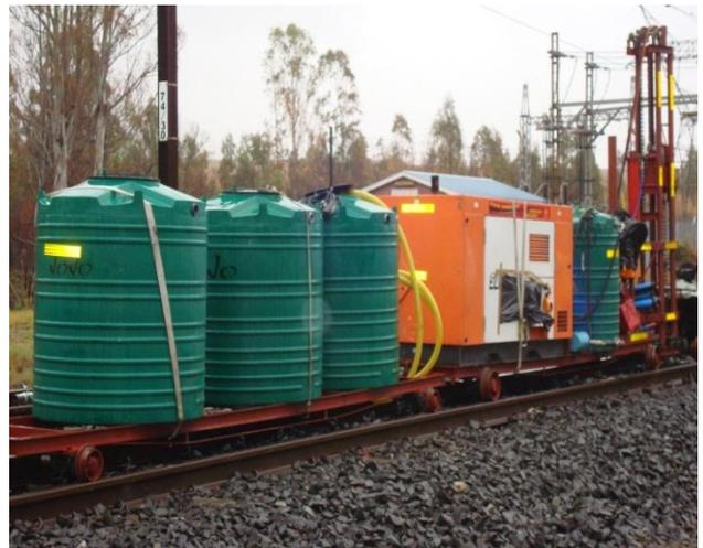
Figure 1: Tailor-made equipment for coring
