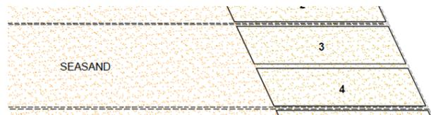
**Figure 5: Geotextile Wrapped around two GSCs and tied back into backfill on the upper layer**
