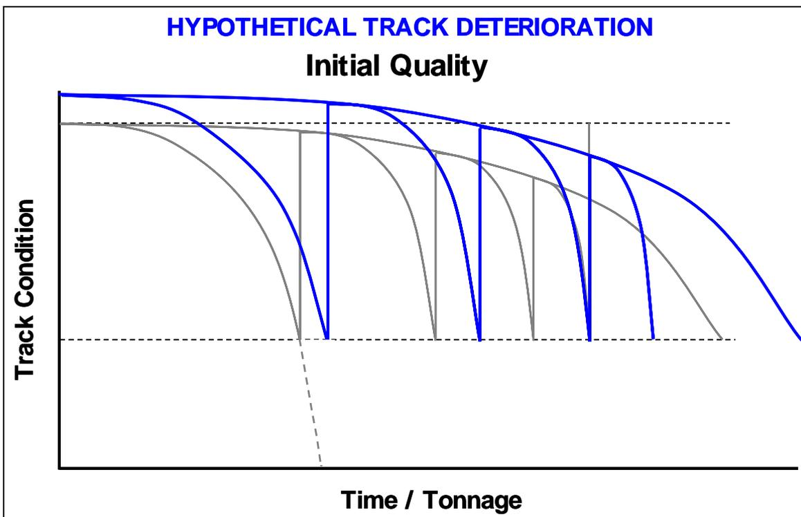
Figure 3 : The Effect Of High Initial Quality On Track Life
