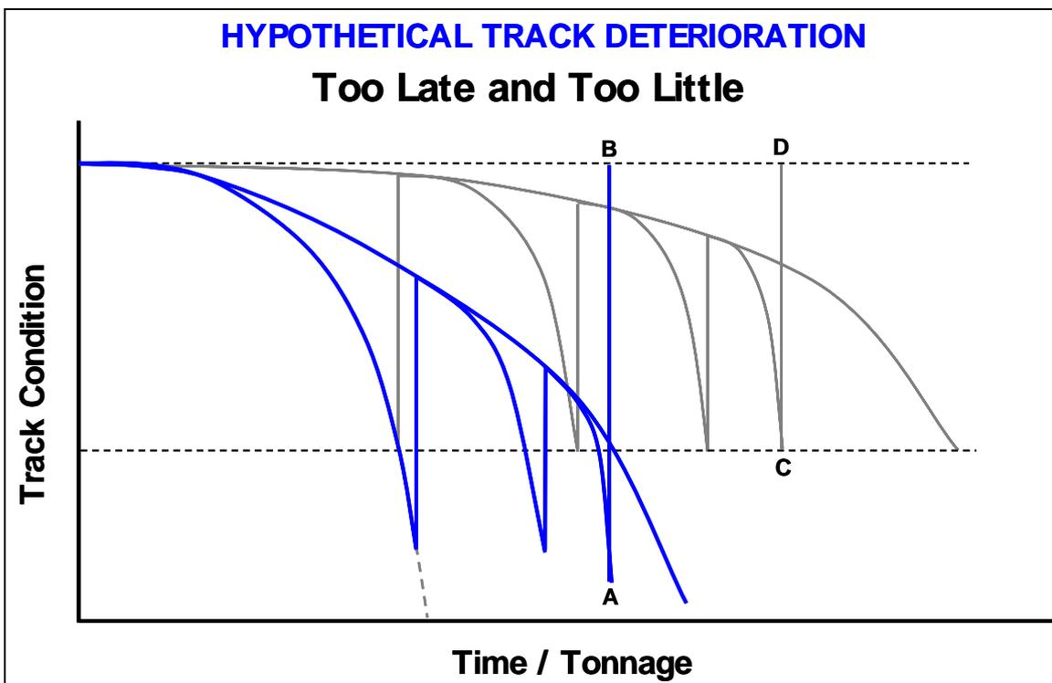
Figure 2 : Track Deterioration Curve With Inadequate Financial Investment
