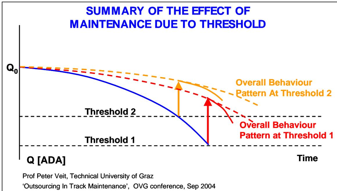
Figure 5 : Summary Of The Effect Of Maintenance Due To Threshold
