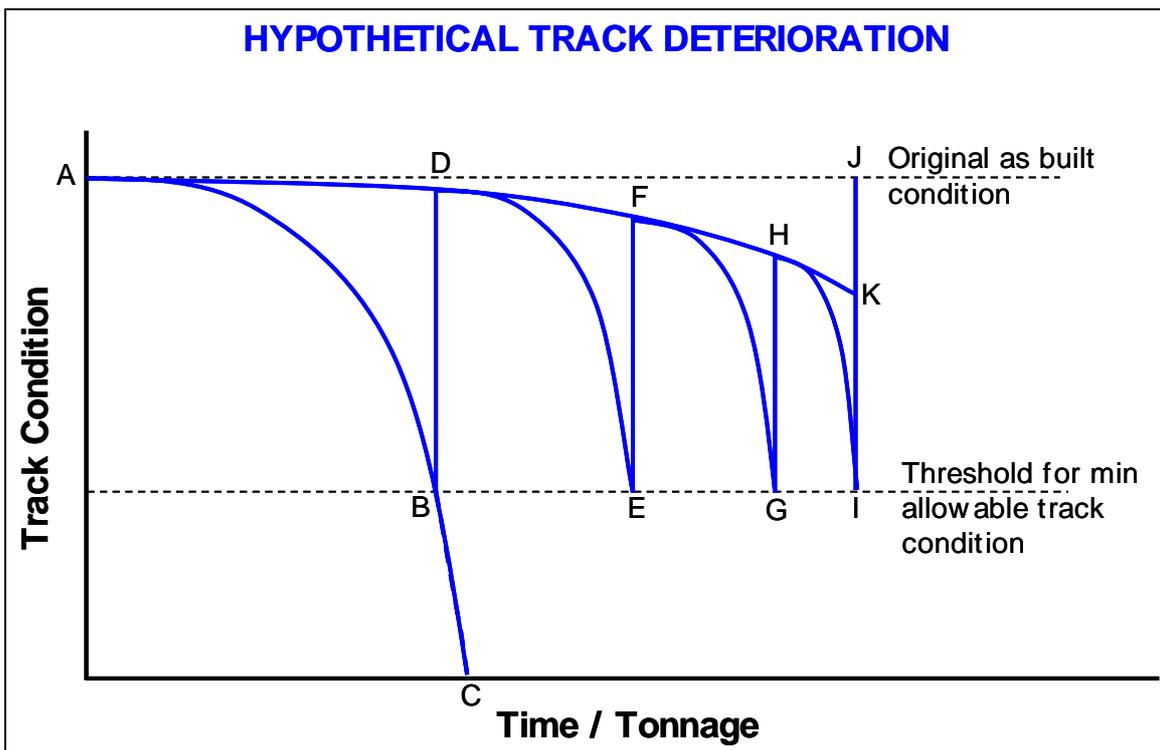
Figure 1 :The Effect Of Maintenance On Track Life
