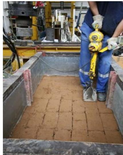
**Figure 4: Clay sub-grade being placed and compacted, Czech Technical University, Prague, 2009**
