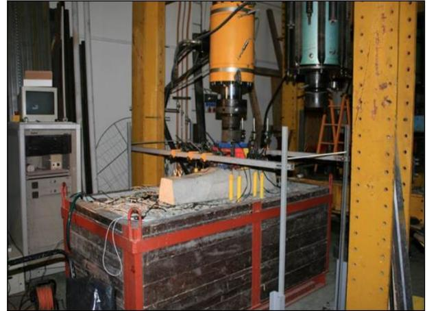
Figure 7: Completed tests section showing sleeper and rail section under load actuator, Czech Technical University, Prague
