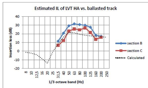
Figure 5. Insertion lost measured/calculated
