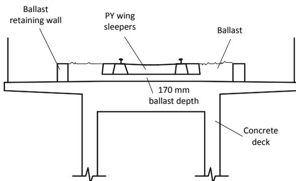
Figure 4. Olifants river bridge cross-section
