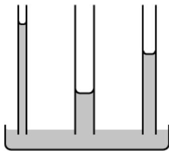
Capillary action tends to collapse the capillary
